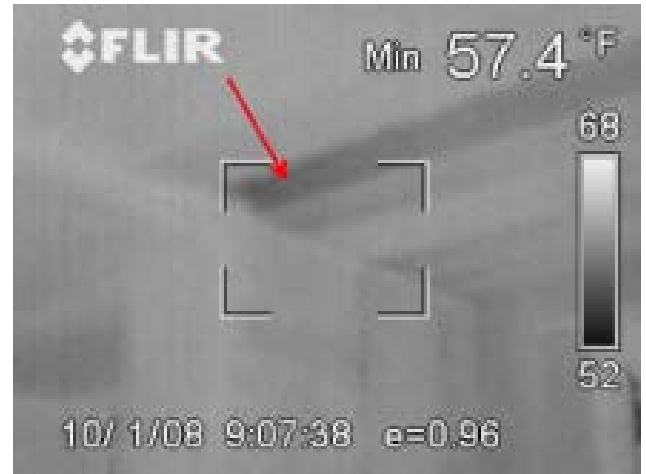
Floor open to outside as shown with cold streak.
